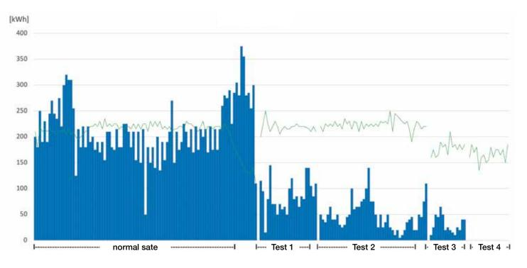
Comparison of the demand for additional heating energy using a conventional cleaner (competitor product/normal condition) and after using eska®phor 7186-1 with determination of optimal process parameters within the scope of four test series.
