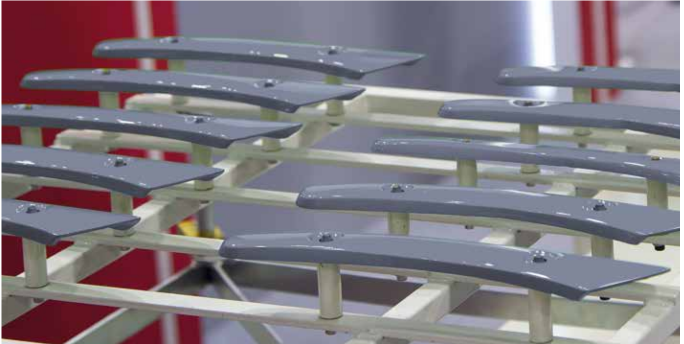
Semi-automated wet painting of plastic parts
